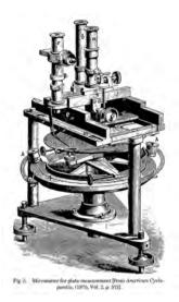
Fig. 2: Lewis Morris Rutherfurd's Photographic Plate Measuring Machine, from entry for 'Micrometer,' in *American Cyclopædia*, vol. 2, New York, 1875, p. 512.
