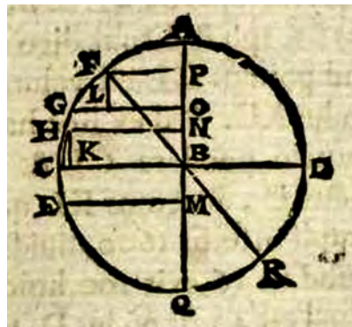
Figure 5.8: According to Cardano, there are three ways to determine positional heaviness. The positional heaviness at point F , for instance, may be determined by the horizontal FP , by the vertical FL , or by the angle QBF . (Max Planck Institute for the History of Science, Library)
